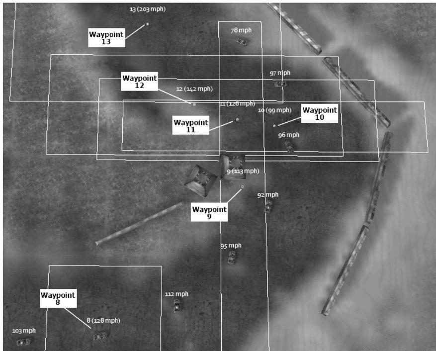
**Fig. 1.** An evolved set of racing waypoints on a dusty tarmac surface. The car aims for the centre of each waypoint (numbered 8 through 13) while targeting the waypoint's indicated speed. As soon as the boundary of a waypoint is crossed, the proceeding waypoint becomes the target. The position, size, and target speeds of the waypoints are evolved using a GA. The position and speed of a car over a period of 8 seconds of the game is illustrated.
